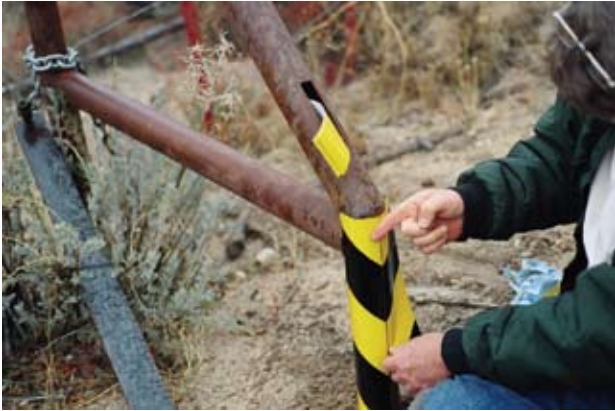
Figure B3. Wrap the yellow and black sheeting around the pipe pointing to the center of the trail.
